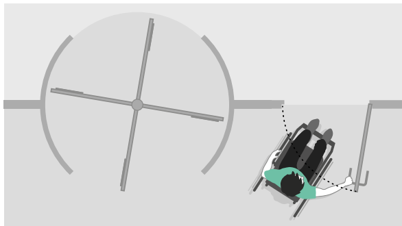
Hinged or sliding doors as an alternative to revolving doors.
