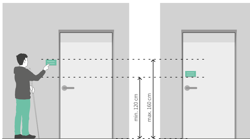
Arrangement principle for Braille information.
