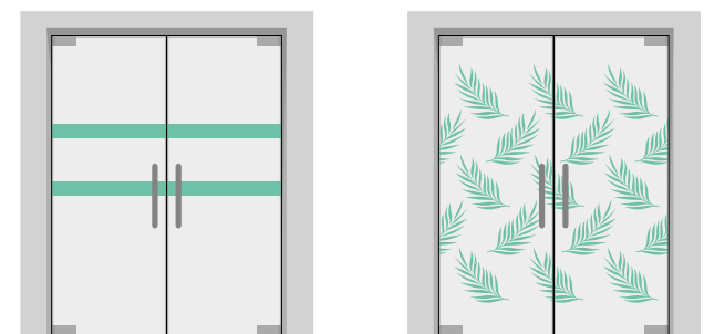
Marking examples of partitions and transparent walls.
